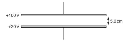
What is the force experienced by an electron in the electric field between the plates?
