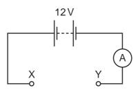
The following combinations of resistors are placed in turn between the terminals X and Y of the circuit.
